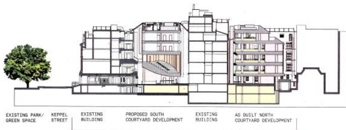
1. Longitudinal section showing the courtyards' new buildings
